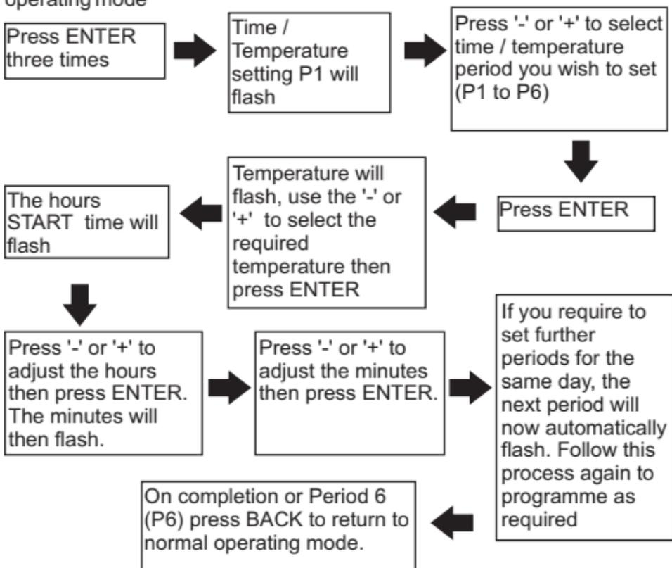
If only two different temperature settings are required in 24 hours then set the first time and temperature using programme one (P1) and the second time and temperature setting using programme setting two (P2). The remaining programmes (P3 to P6) should all be set to the same time and temperature as P2.
