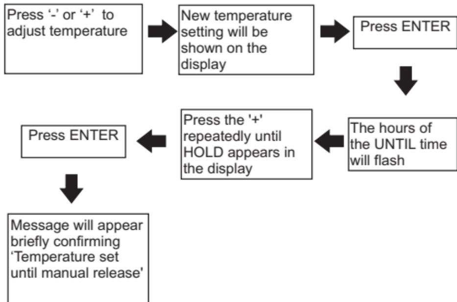
In the 'HOLD' position the temperature can be overridden by pressing either the '-' or '+' . This will then become the new 'HOLD' temperature
